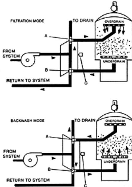
Five percent of 1200 gpm is 60 gpm, which requires a 24-inch filter with a flow rate of 63 gpm.
